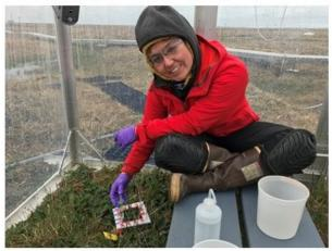
**Figure 2.** A Zero-Power Warming (ZPW) chamber. The chamber is warmed passively by solar radiation. The combination of an internal and an external heat exchanger modulates venting of the chamber, which enables the air temperature to be elevated by about 4°C.
