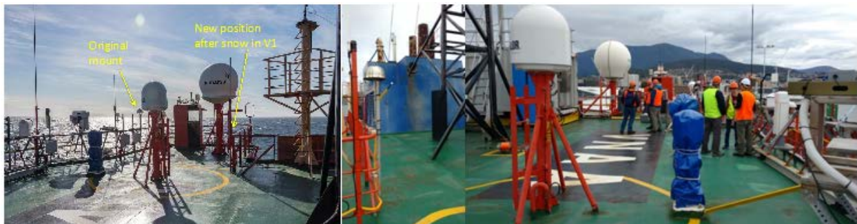
Figure 1. Instrumentation and filter positioning on the Aurora Australis . Left: the original mount of the filter unit (globe is a rain hat) along the front rail of the upper deck with other instruments. This position was problematic in snow situations. Middle: The mounting position after snow filled the rain hat during a storm in voyage 1 (V1). The ship stack is in the blue building structure to the aft. Right: View from the final filter position across the deck, with the AOS trailer (blue) just visible on the far-left side of the view.
