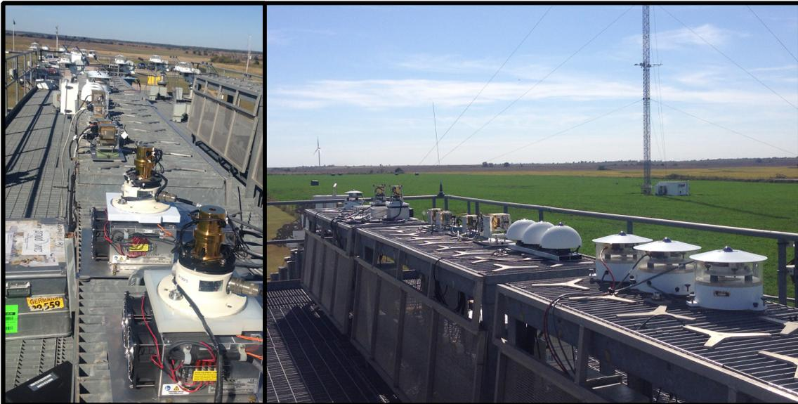
**Figure 1.** Deployment of infrared standard instruments for intercomparisons at the SGP calibration facility in the fall of 2018. Two ACP can be seen in the foreground at left with four IRIS instruments just behind. At right, the PIRs tied to the WISG from Davos are positioned next to the IRIS followed by the three PIRs held by the National Oceanic and Atmospheric Administration (NOAA) that were also tied to the WISG.
