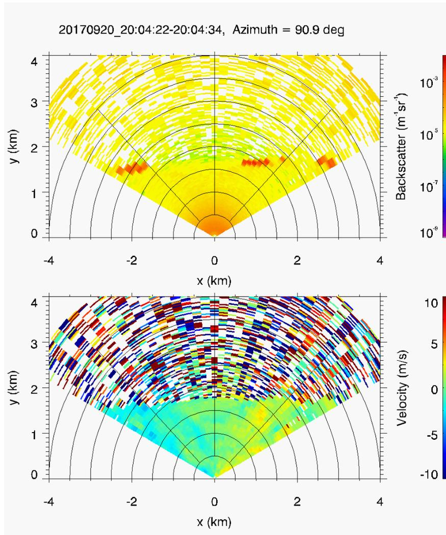
**Figure 1.** Observed FWC with Doppler lidar cross-wind RHI scan on September 20, 2017. Upper panel: Doppler lidar backscatter. Lower panel: Doppler lidar radial velocity.
