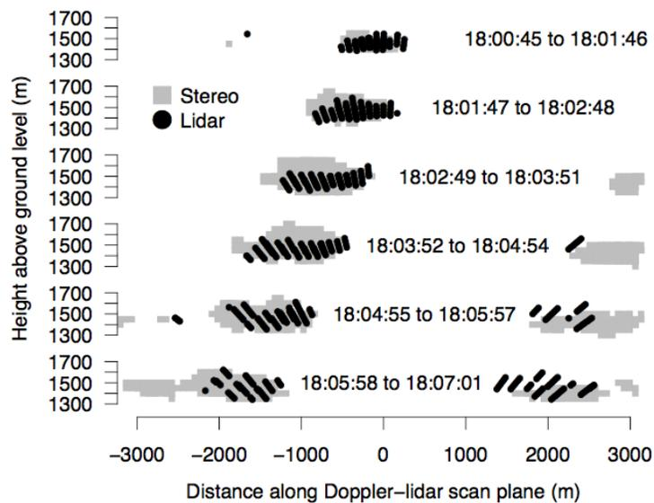
**Figure 3.** A comparison of scanning Doppler lidar cloud detections and stereo camera cloud points in the same plane as the Doppler lidar scan on August 31, 2017.
