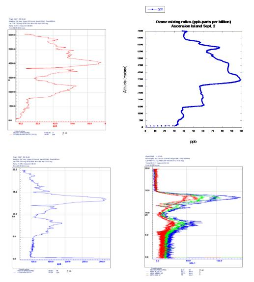
Figure 2. Top: Aircraft ozone mixing and ground-based ozone mixing ratios; Bottom: Aircraft CO mixing ratios and aerosol measurements.
