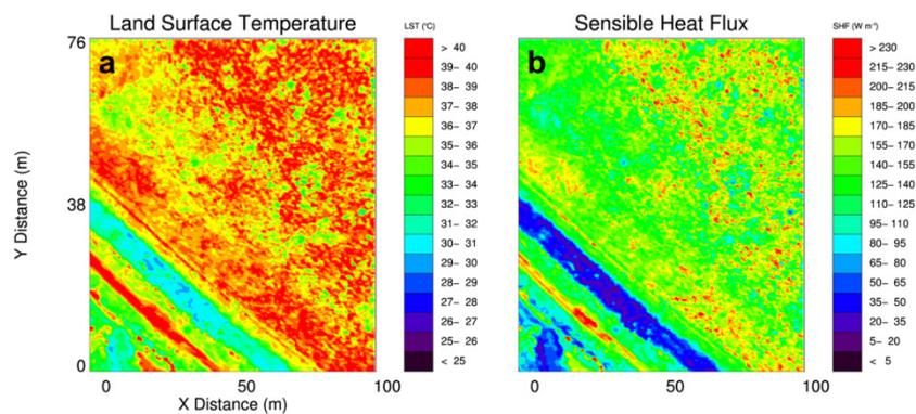
**Figure 3.** Example of heterogeneity in LST (a) and sensible heat flux (b), determined from the infrared camera during the DJI S-1000 sUAS flight at 1943 UTC on 17 August, 2017.
