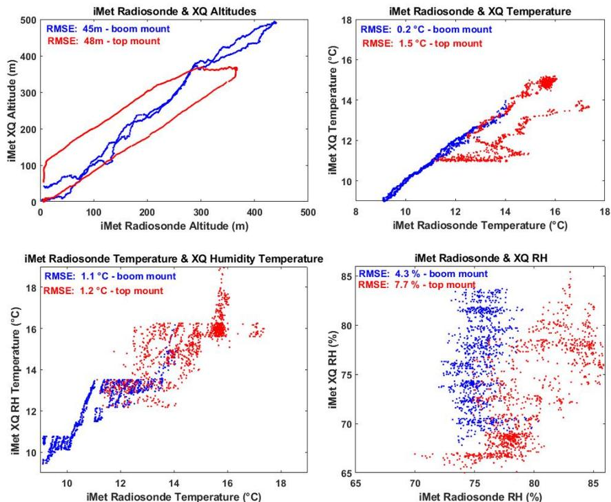
**Figure 3.** Comparison of iMet radiosonde and iMet-XQ UAV sensor measurements when iMet-XQ sensor was mounted along the UAV boom or on top of the UAV.
