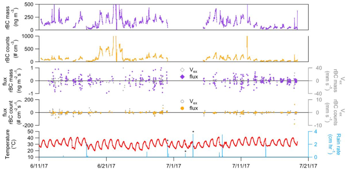
**Figure 3.** Campaign overview of rBC mass, particle counts, fluxes, vertical exchange, and several meteorological parameters. Flux periods shown are all possible flux periods and have not been quality controlled. Data presented subsequently represents quality-controlled data. Rain periods marked with an (\*) refer to periods of collected precipitation. Rain rates were measured using a weighing bucket precipitation gauge (ARM Climate Research Facility, Weighing Bucket Precipitation Gauge).
