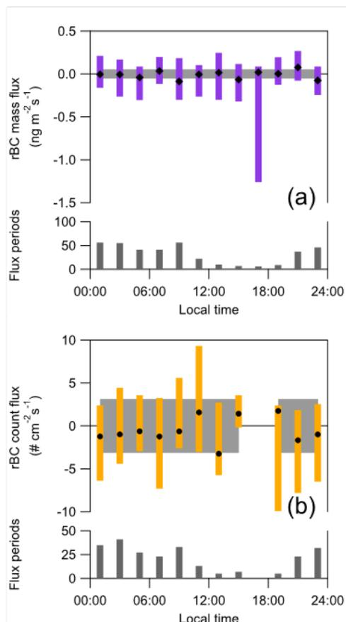
**Figure 4.** Bi-hourly binned fluxes of rBC counts (a) and rBC mass (b). Symbols are medians; upper and lower ends of the boxes are the 75th and the 25th percentiles respectively. The shaded grey bar represent the length of day (LOD), and bottom vertical bars are the number of flux periods that represent the data above.
