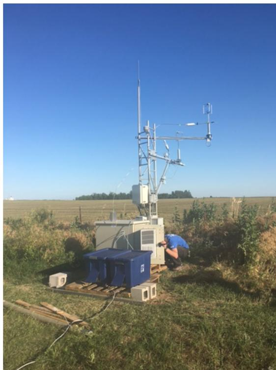
**Figure 1.** Instrument set-up for BCADS 2017. The blue boxes housed the pumps, and the air conditioned box housed the SP2) and UHSAS.
