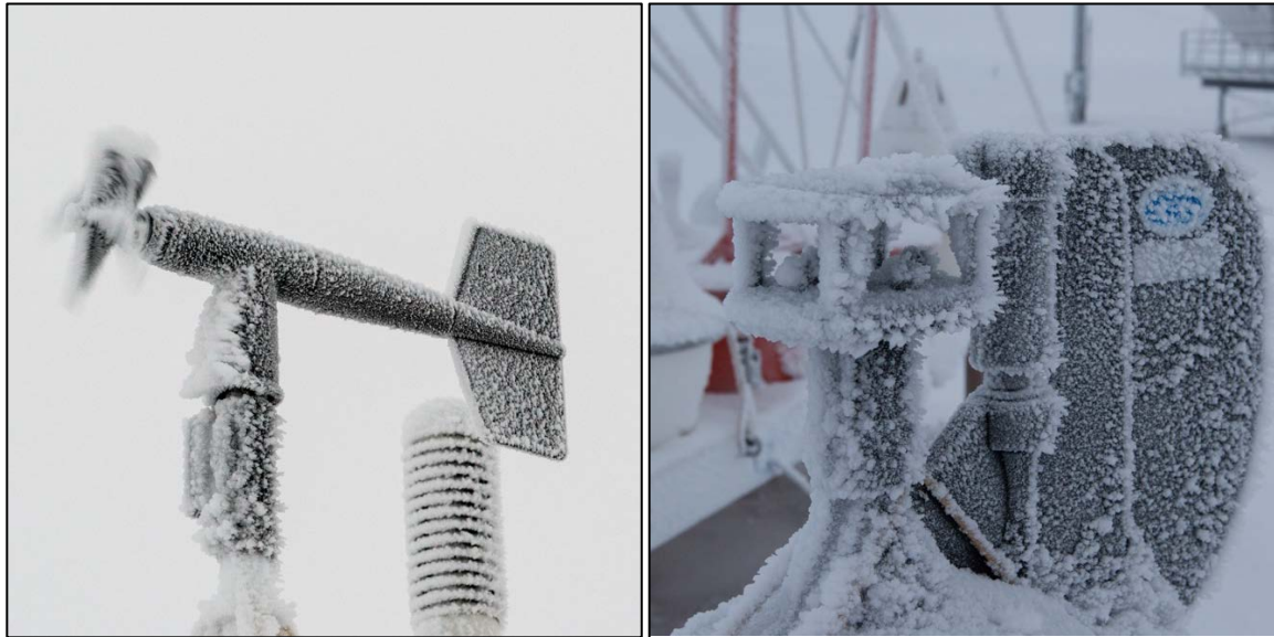
Figure 3. Winds at the test site were obstructed by the buoys on the test bed and by buildings of the ARM (west, Figure 1) and NOAA/CMDL (east) sites. From the unobstructed wind directions, the buoys compared to the CMDL winds had a slow bias of 0.8 m/s with an RMS difference of ~1.4 m/s. These differences were greater during periods when the anemometer was frosted, and even frozen up for two weeks as pictured above. The ultrasonic anemometers tested were more susceptible to frost.
