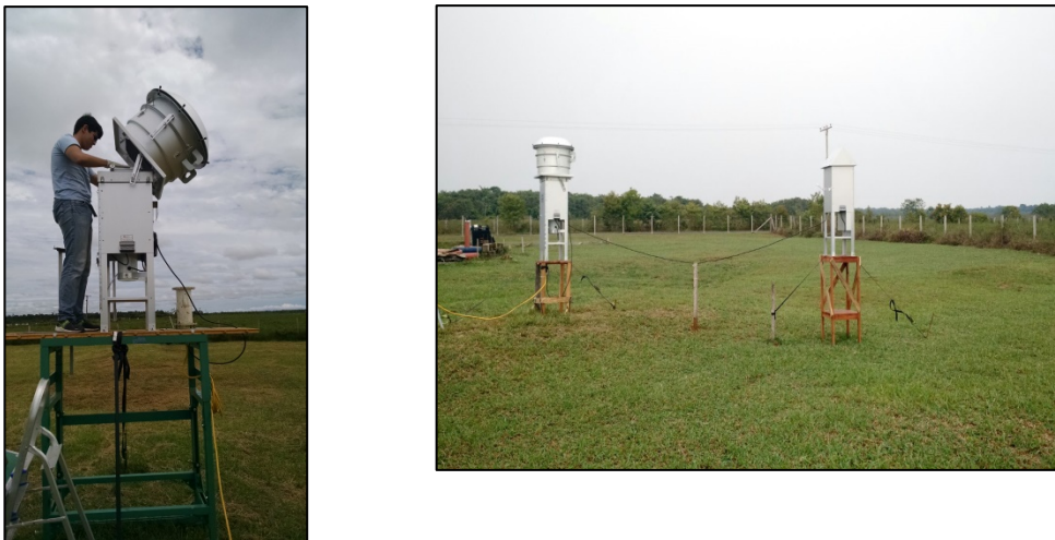
Figure 1: High-volume samplers ( \text{PM}_{2.5} and TSP) at the ARM site in Manacapuru, Amazonas.
