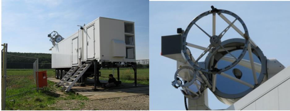
**Figure 11.** The UHOH 3D scanning WV DIAL. Left: Mobile trailer. Right: 80-cm 3D scanner.
