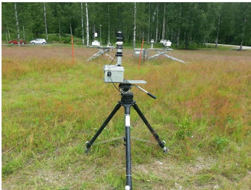
**Figure 1.** TWST optical head as deployed during BAECC.
