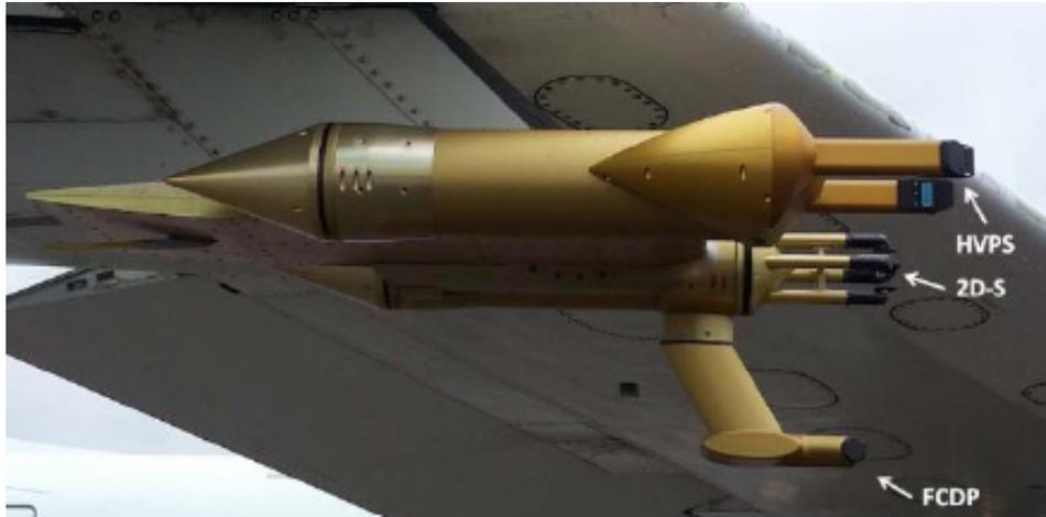
**Figure 1.** SPEC, Inc. instruments installed on the NASA DC-8 during SEAC4RS.
