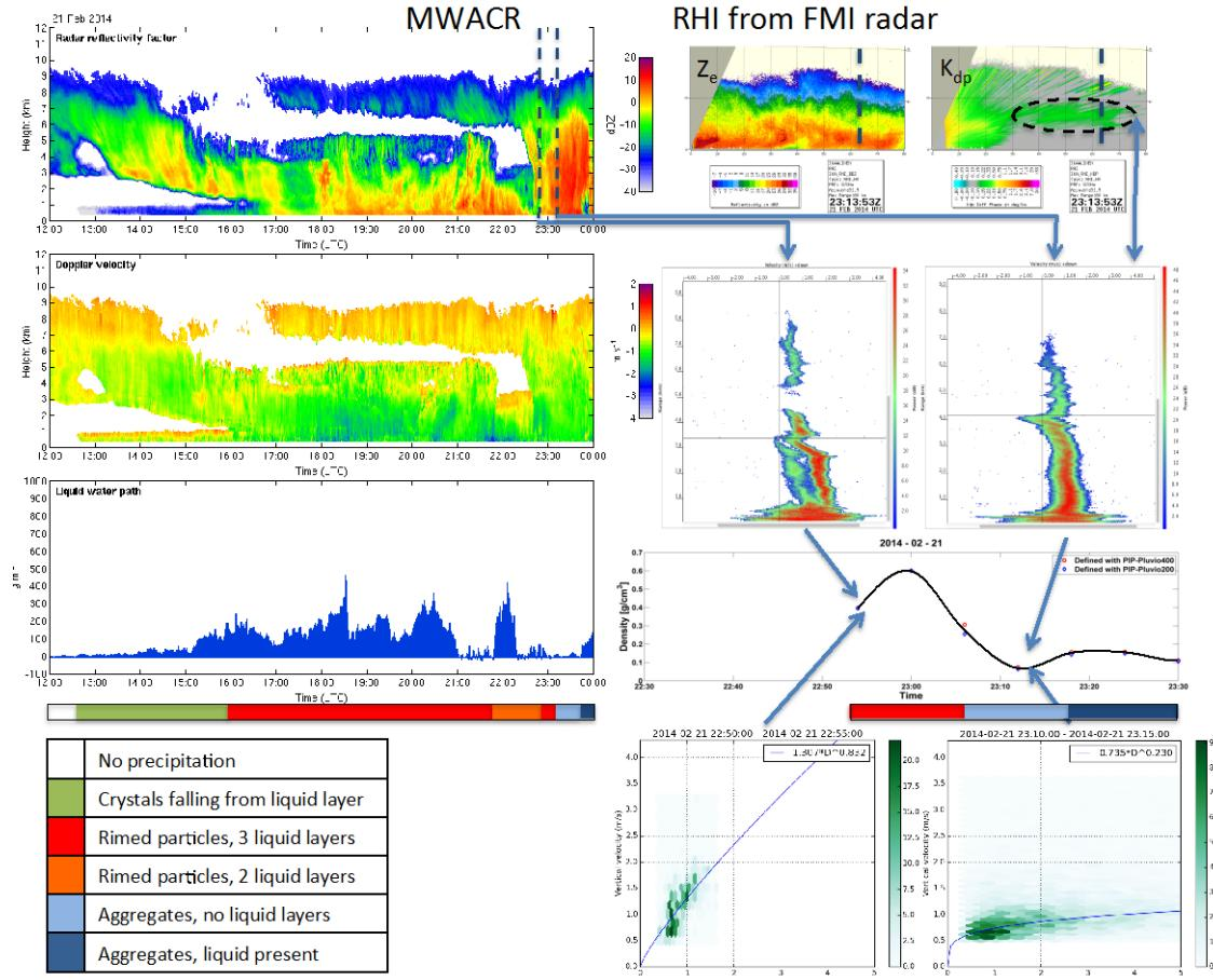
**Figure 17.** An example of application of cloud radar, Doppler radar spectra, surface precipitation observations, and scanning dual-polarization radar to characterize dominating precipitation processes. Measurements were collected on February 21, 2014 during BAECC SNEX IOP. FMI radar carried out RHI scans over the AMF2 location every 15 min.
