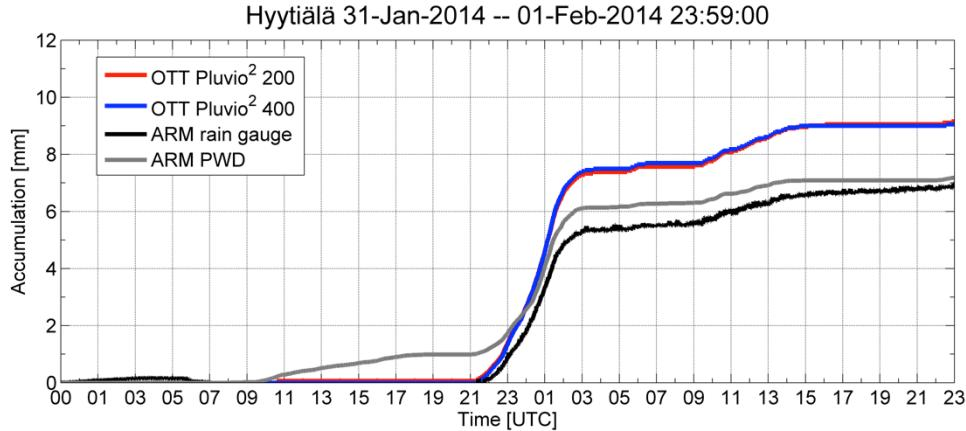
**Figure 16.** An example of precipitation accumulations measured by two University of Helsinki gauges (OTT Pluvio<sup>2</sup> 200 and 400) and ARM weighing gauge and PWD. Measurements were collected on February 1, 2014 during BAECC SNEX IOP. The OTT Pluvio<sup>2</sup> 200 gauge is located inside of DFIR and OTT Pluvio<sup>2</sup> 400 is located outside.
