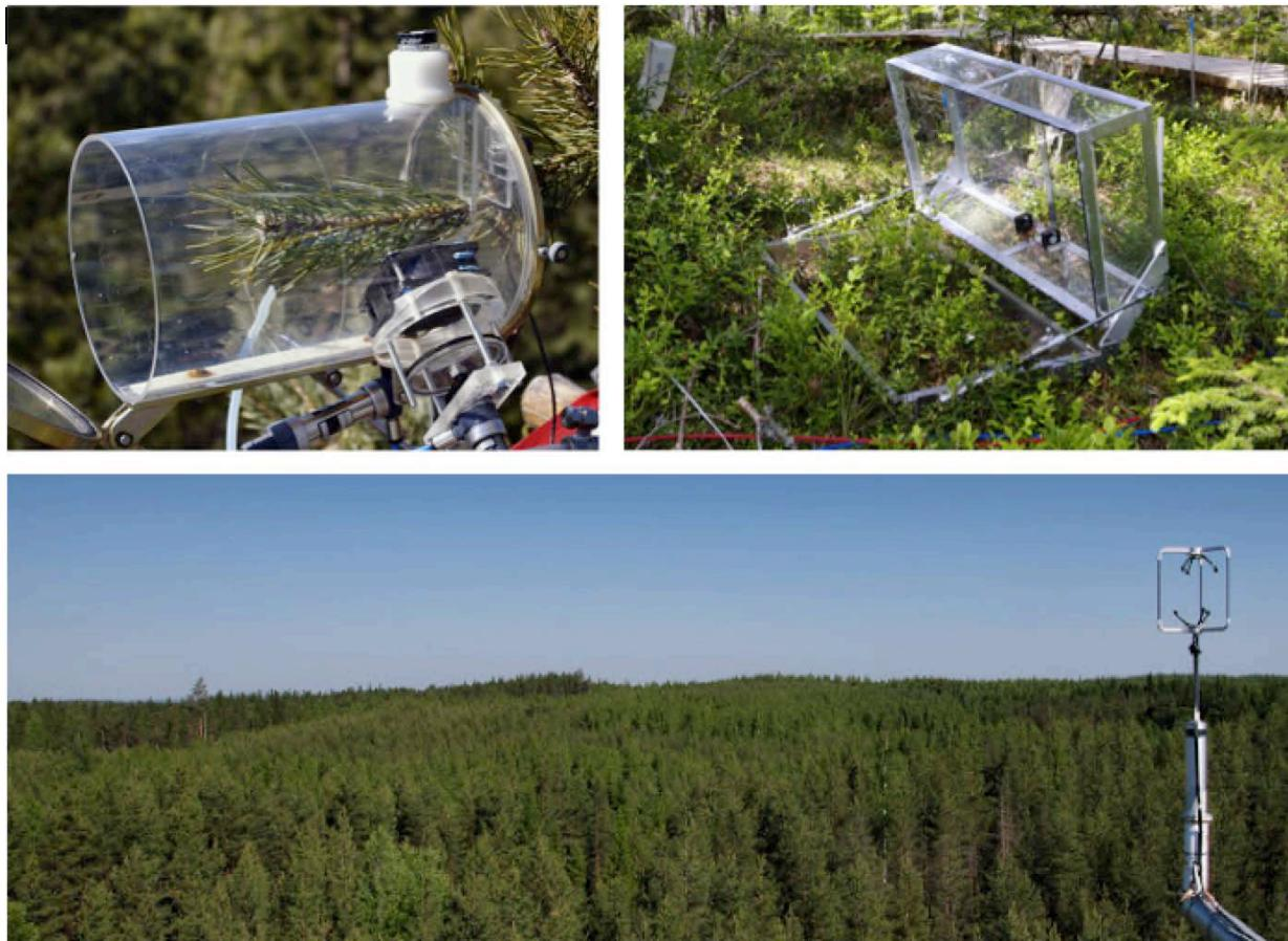
**Figure 4.** The emission of biogenic volatile organic compounds (BVOCs) were determined using branch cuvettes (top left) and soil chambers (top right). Eddy covariance technique together with fast response Proton Transfer Reaction Mass Spectrometer (PTR-MS) (Taipale et al., 2011) allows us to determine ecosystem scale fluxes (bottom).
