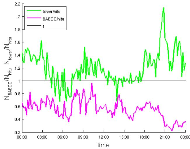
**Figure 6.** Fraction of tower- and BAECC-DMPS compared to SMEAR-DMPS for 6 to 25 nm nucleation mode particles. Comparison is carried out for diurnal median concentrations for event days between March and August 2014.
