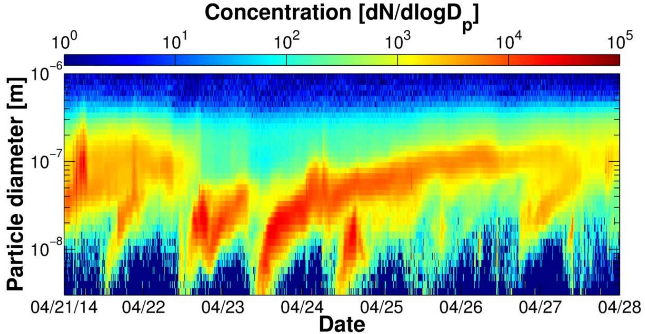
**Figure 2.** Sub-micron aerosol number size distribution measured with a SMEAR-II Differential Mobility Particle Sizer (DMPS) at Hyytiälä, Finland between 21 and 27 April, 2014 featuring the characteristic phenomenon observed at the site: formation of secondary organic aerosol and their growth to CCN active sizes.
