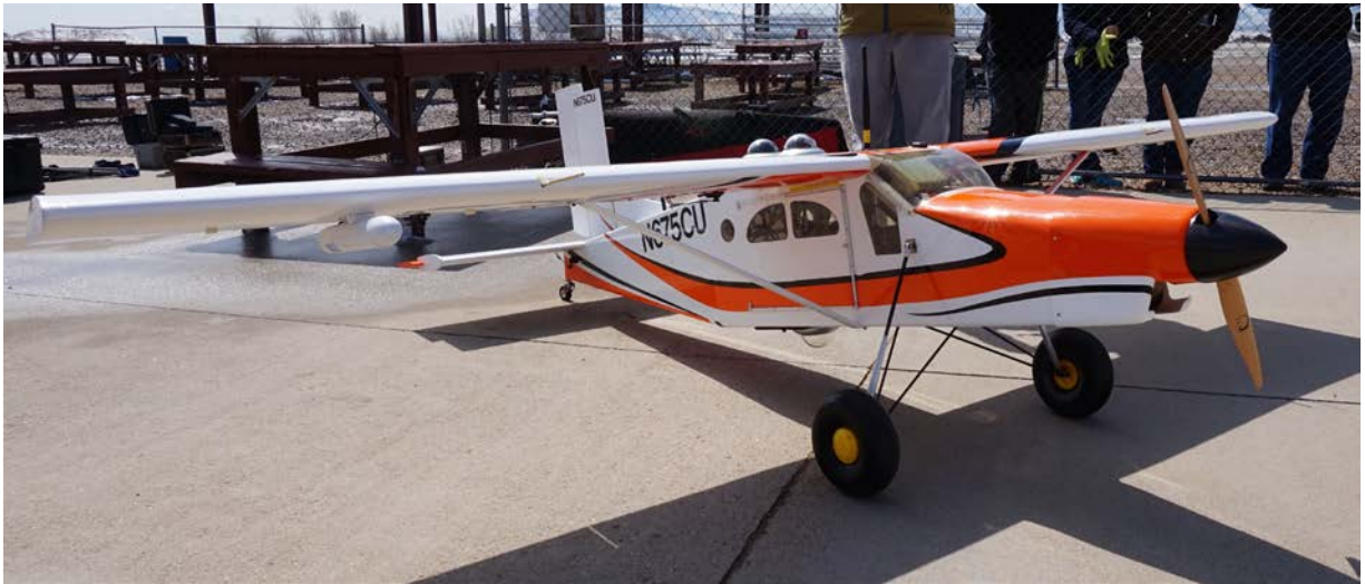
Figure 2. The Pilatus UAS shown equipped with the PTH module (white, on wing), SPN-1 Shortwave Pyranometers (two upward and one downward looking), and the POPS Aerosol Spectrometer (in windshield).
