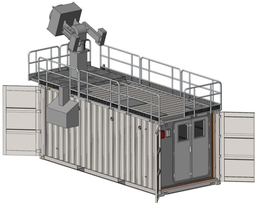
**Figure 2.** Depiction of the OPS van to be located at the Thunderhead Lodge. SWACR is mounted on the roof at one end and AERI enclosure can be seen mounted to side of van. Portholes in roof for high spectral resolution lidar and MPL are located on near side. The MFRSR, MWR, and IRT will be located roughly at top of railing at end opposite the SWACR.
