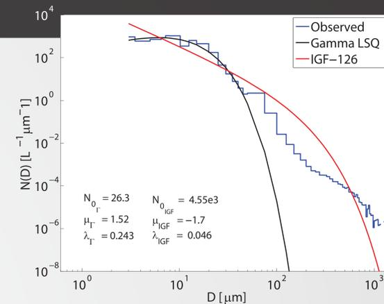
Figure 1: IGF method and standard least squares fit applied to a 60 s PSD measured 0805-0806 UTC on 29 Jan 2006 during TWP-ICE.
