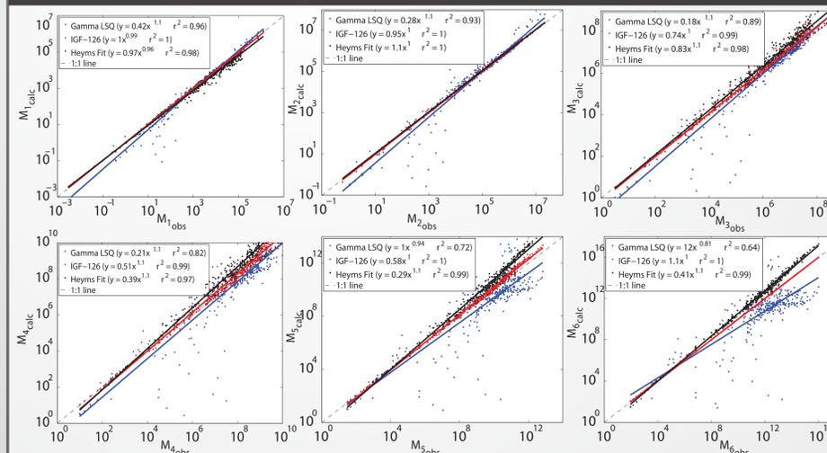
Figure 2: Comparisons of moments calculated from observed PSDs,  $M_{x_{obs}}$ , against moments calculated from fit distributions,  $M_{x_{calc}}$ , for moments 1 through 6.
