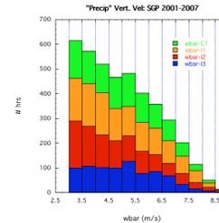
During rainfall events, scattering from raindrops overwhelms atmospheric scattering. We roughly related fall velocity ( $w_d$ ) and droplet size ( $D$ ) as  $D = .27e^{(.304w_d)}$  in order to estimate rainfall. Only hourly averaged vertical velocities greater than 3 m/s were included.
