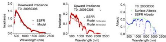
C) T2 supersite is located approx. 60 km NE (downwind) of T0 on private ranch land (parched grass). J-31 aircraft was 3810 m AGL when this data was taken. Mean aerosol properties between plane and ground were measured using an Aeronet sunphotometer [5] and a PSAP/nephelometer [4].
