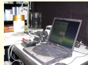
Dynamic rain gauge calibrator developed through a collaborative effort between the University of Iowa and ARM.
