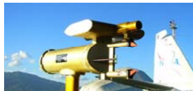
FIG 4: Picture of CAS as installed on WB-77 during CR-AVE, January 2006. Inlet, but not shroud, present.
