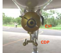
FIG 3: Cloud Droplet Probe (CDP) that sizes between 2 and 50 \mu\text{m} , and Counterflow Virtual Impactor (CVI) that provides bulk measures of mass.
