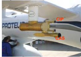
FIG 2: Cloud Aerosol and Spectrometer Probe (CAS) that sizes between 0.5 and 50 \mu\text{m} , and Cloud Imaging Probe (CIP) that nominally sizes between 25 and 1550 \mu\text{m} .
