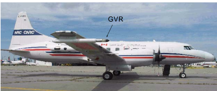
Figure 2. In September 2006 the Airborne GVR was installed in the NRC Canada Convair-580 Aircraft to participate in the CloudSat validation flights.
