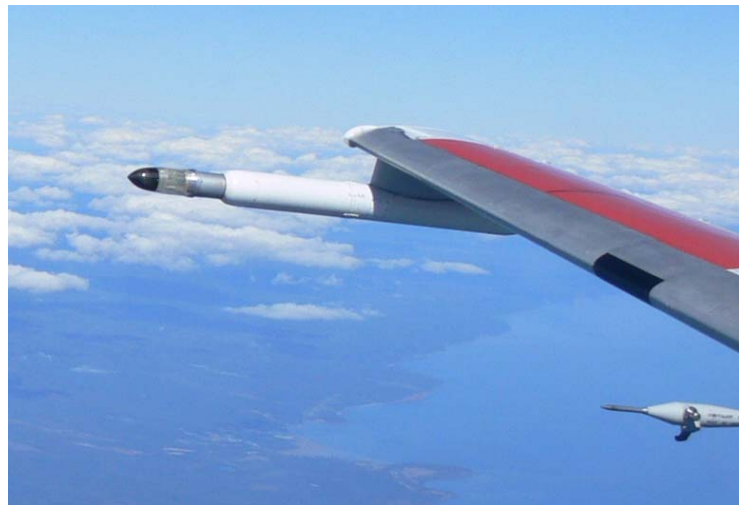
Figure 3. On the NRC Convair-580 Aircraft, GVR was installed in one of the outside PMS probe pods, so the Zenith pointed antenna beam would clear the wing.
