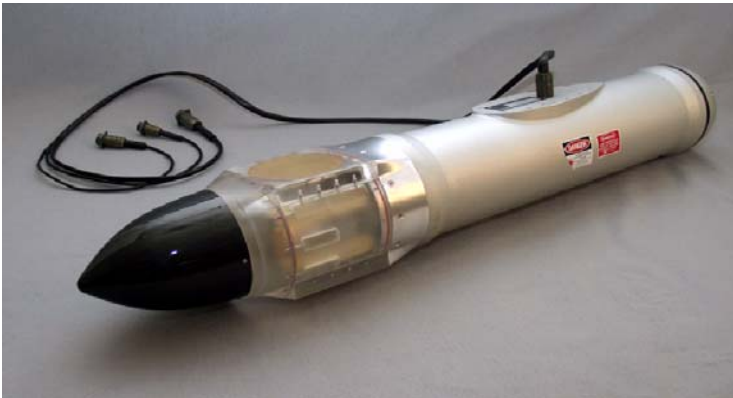
Figure 1. Airborne GVR, packaged and wired to operate from a standard PMS probe canister. A sampling rate of about 10 Hz is interrupted with a 0.25 sec calibration gap once every three seconds. Instrument weight is 22 lb; 38 lb total as shown installed in a PMS 2-D probe canister.
