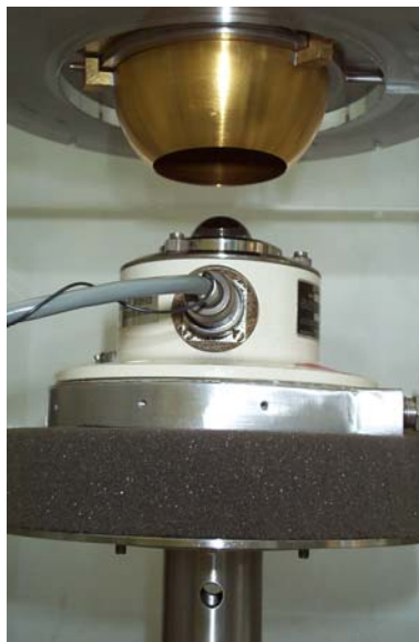
Figure 3b. Close-up of PIR beneath blackbody completion hemisphere. PIR dome is fully inserted during calibration data acquisition.
