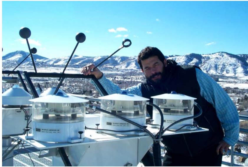
Figure 1a. Three Eppley Model precision infrared radiometer (PIR) pyrometers mounted in ventilators on a solar tracker to provide shading of direct shortwave (solar) radiation. Each PIR has a thermopile detector under a protective hemispheric interference filter transparent to longwave radiation (3.5 to 50 microns).
