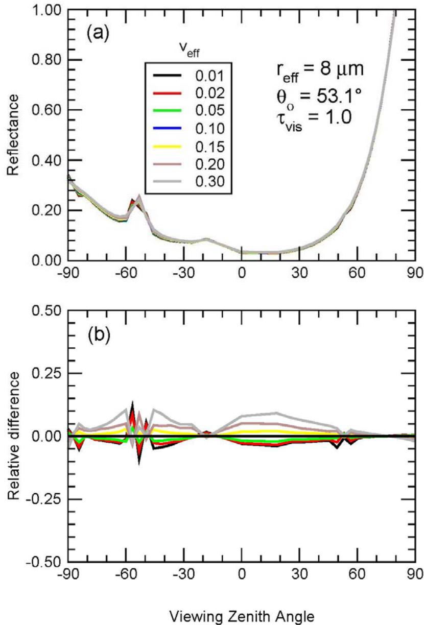
**Figure 4.** Cloud reflectance at 0.65  $\mu\text{m}$  for a typical satellite observation. (a) reflectance in the principal plane and (b) relative difference with respect to  $v_{\text{eff}} = 0.10$ .
