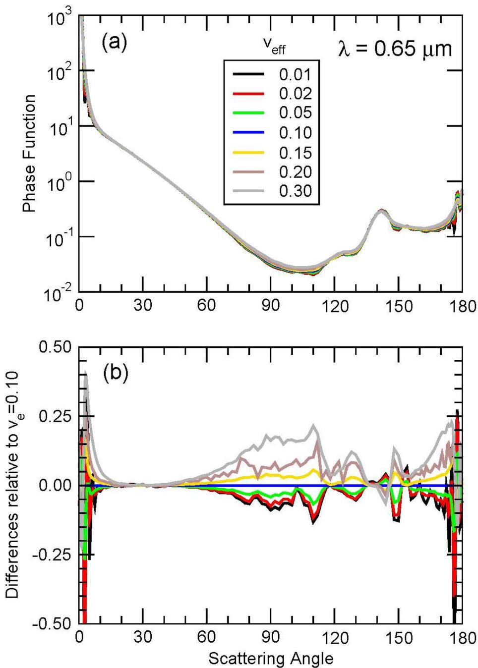
**Figure 2.** Scattering phase function for  $r_{\text{eff}} = 8 \mu\text{m}$  at  $0.65 \mu\text{m}$ . (a) phase function and (b) differences in phase function due to  $v_{\text{eff}}$  relative to  $v_{\text{eff}} = 0.10$ .
