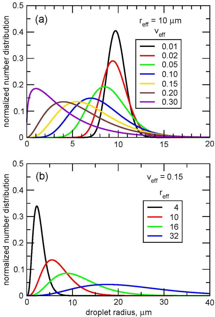
**Figure 1.** Normalized modified  $\Gamma$ -distributions used in this study, showing (a) the effect of the parameter  $v_{\text{eff}}$  for a given  $r_{\text{eff}}$  and (b) the effect of  $r_{\text{eff}}$  for a given  $v_{\text{eff}}$ .
