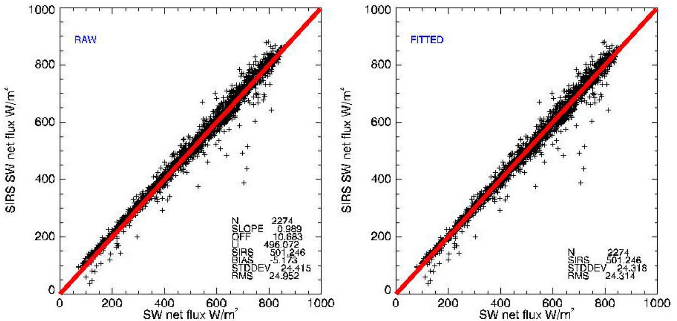
**Figure 1.** Clear-sky daytime surface SW net flux from the SIRS instrument and the Li-Leighton method.
