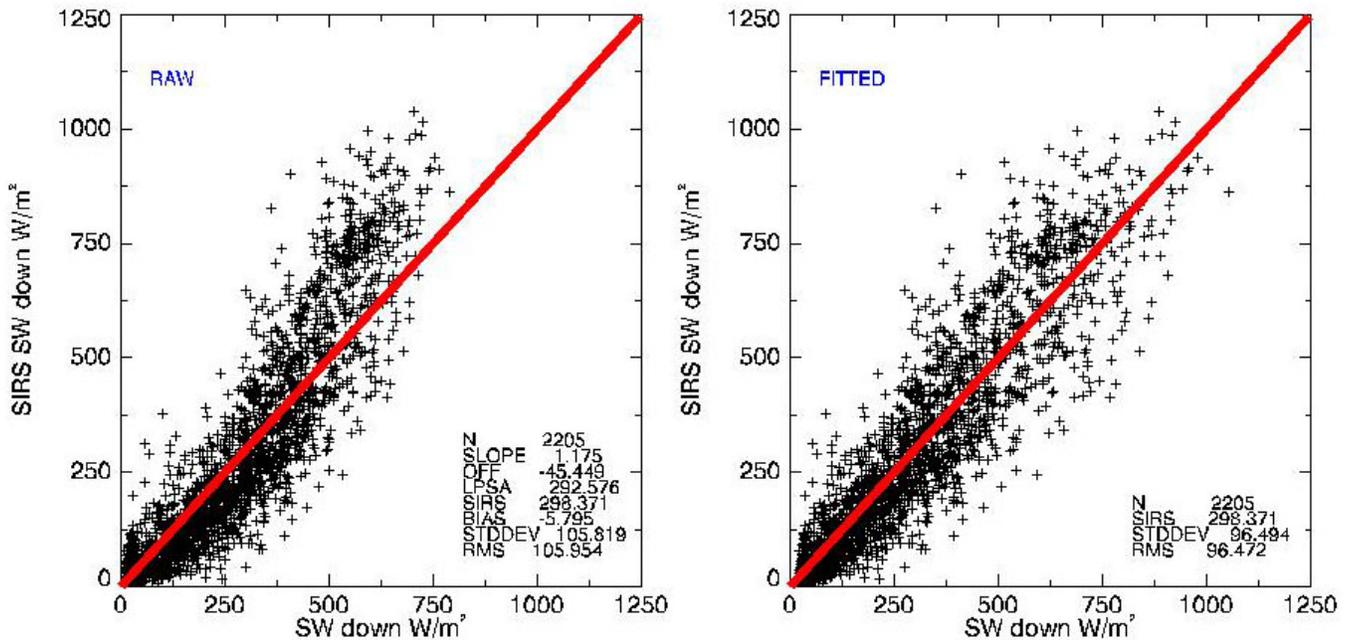
**Figure 5.** Daytime SW downwelling flux under cloudy conditions from SIRS and LPSA.
