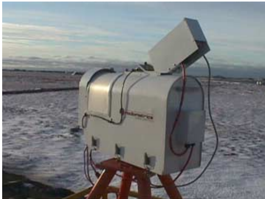
Figure 1. The MWRP deployed at the ARM NSA CF in Barrow, Alaska. The IR (10-micrometer wavelength) thermometer mounted on the MWRP provides an estimate of cloud base temperature, which is used to infer cloud base height and constrain the liquid water content (LWC) retrieval.
