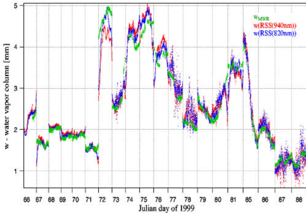
Figure 6. Water vapor column as function of time for 20 concatenated days.
