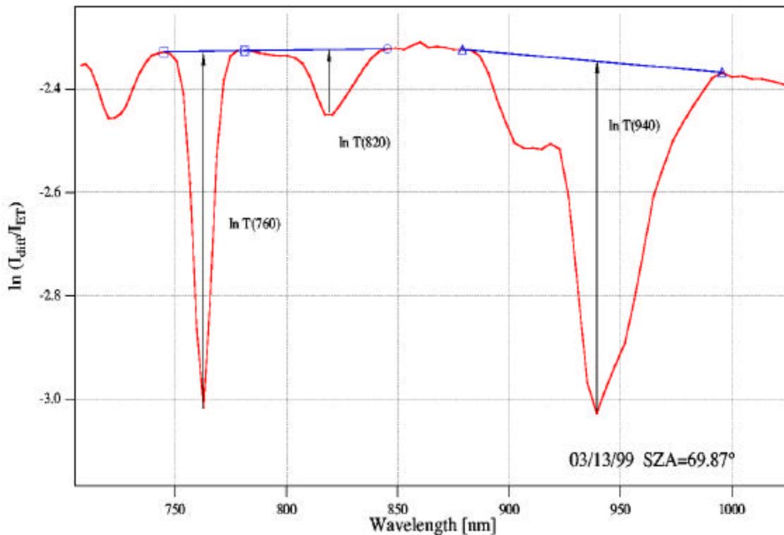
**Figure 2.** Example of diffuse irradiance. The anchor points used to define baselines for each absorption band are marked.
