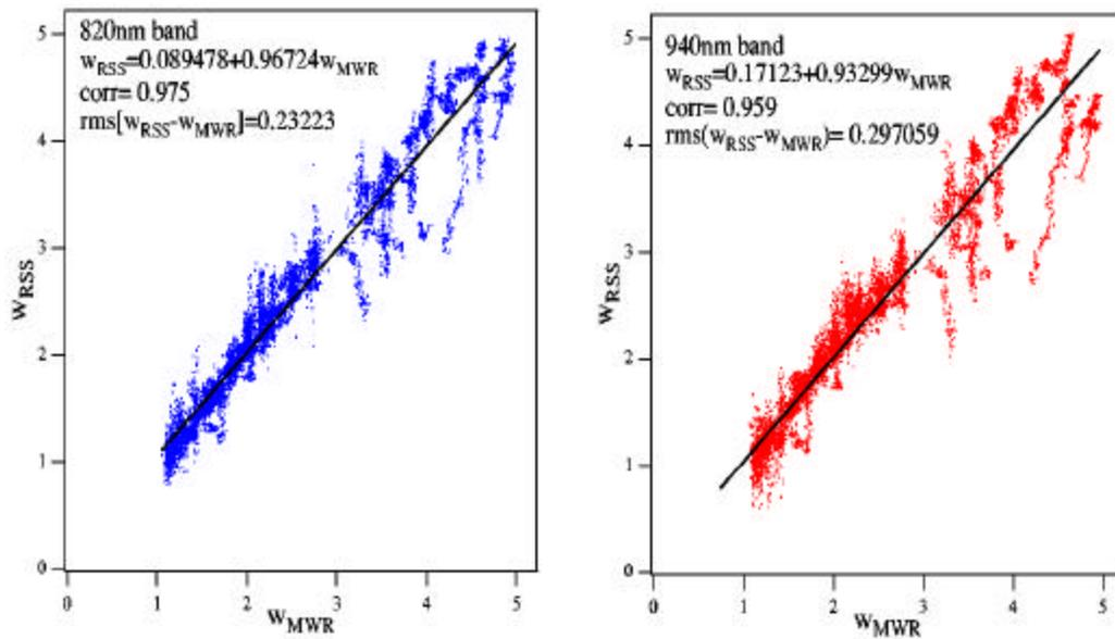
Figure 5. Correlation plots between RSS and MWR retrieved water vapor column.
