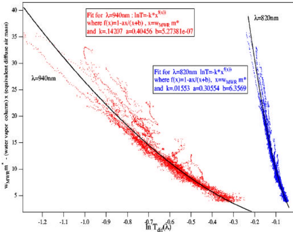
**Figure 4.** Derivation of effective diffuse curves of growth at 820 nm and 940 nm.
