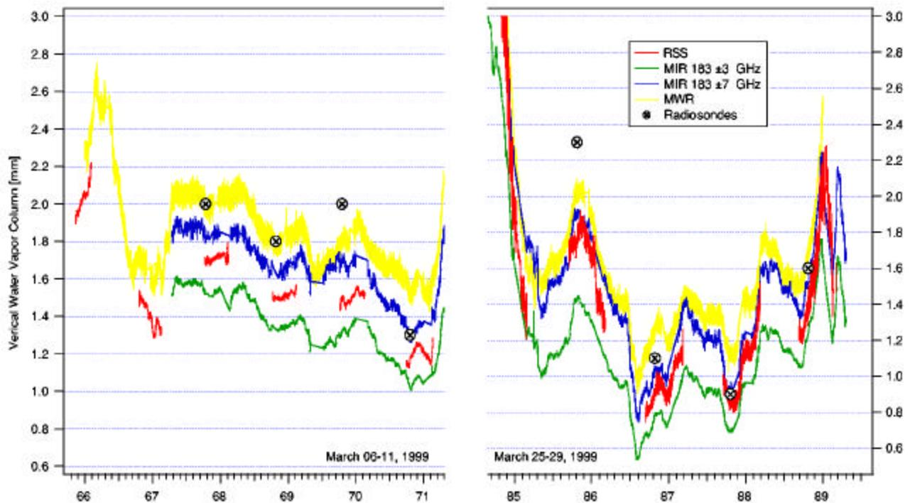
**Figure 1.** Comparison of water vapor retrievals with microwave radiometers and with direct beam RSS data on clear and semi-clear days.
