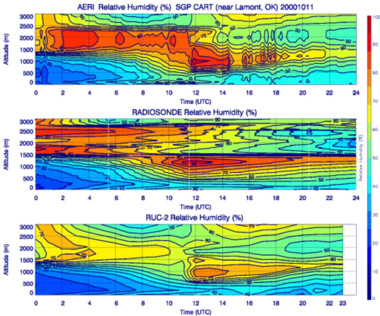
**Figure 2.** Time-height cross sections of RH from the AERI instrument, radiosondes, and RUC-2 numerical weather prediction model on October 11, 2000. The time resolution for the AERI profiles are 10 min, white lines indicate radiosonde launches, and the RUC-2 data is the hourly analysis.
