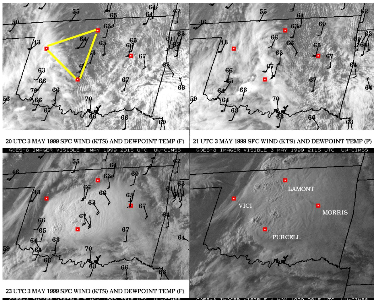
**Figure 3.** GOES-8 visible satellite images from 2000 UTC to 2359 UTC on May 3, 1999, over the ARM SGP CART site domain. The AERI locations are indicated by the red dots. Moisture flux advection and divergence calculations were conducted for the three AERI systems connected by the yellow triangle.
