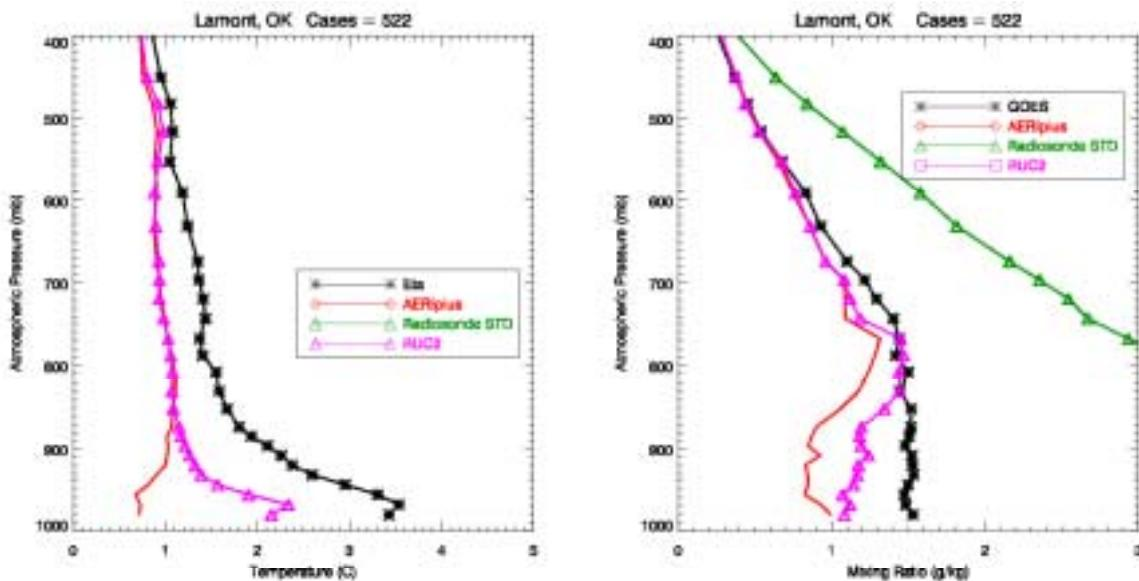
**Figure 1.** Temperature and mixing ratio rms differences compared to 522 Vaisala radiosonde launches compared to Eta (black line), RUC-2 (magenta line), and physically retrieved AERI profiles (red line) for March to December 2000 at the central SGP Cloud and Radiation Testbed (CART) site facility. A green line indicates the radiosonde standard deviation for temperature and mixing ratio during this period if within x-axis domain.
