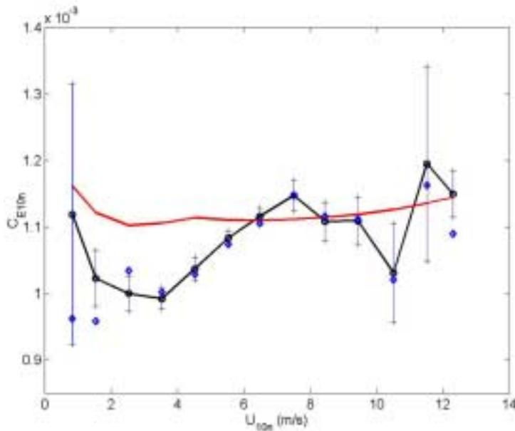
**Figure 4.** 10-m neutral moisture transfer coefficient ( $C_{E10n}$ ) versus 10-m neutral wind speed. The direct measurements are given using medians (circles) and means (diamonds); the red line is COARE Version 2.6. The bars indicate the statistical uncertainty in the mean estimate.
