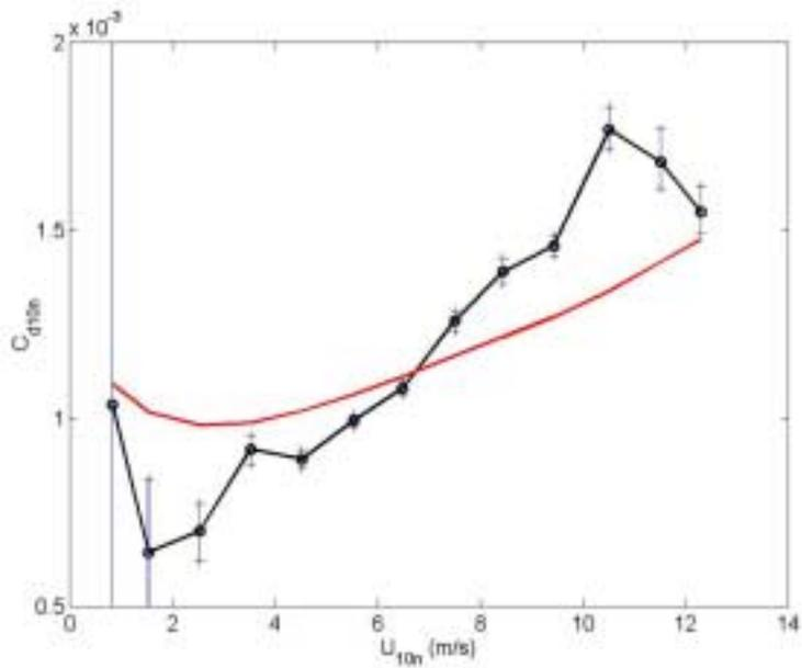
**Figure 5.** 10-m neutral momentum transfer coefficient ( $Cd_{10n}$ ) versus 10-m neutral wind speed. The direct measurements are given using medians of the combined covariance and ID values (circles); the red line is COARE Version 2.6. The bars indicate the statistical uncertainty in the mean estimate.
