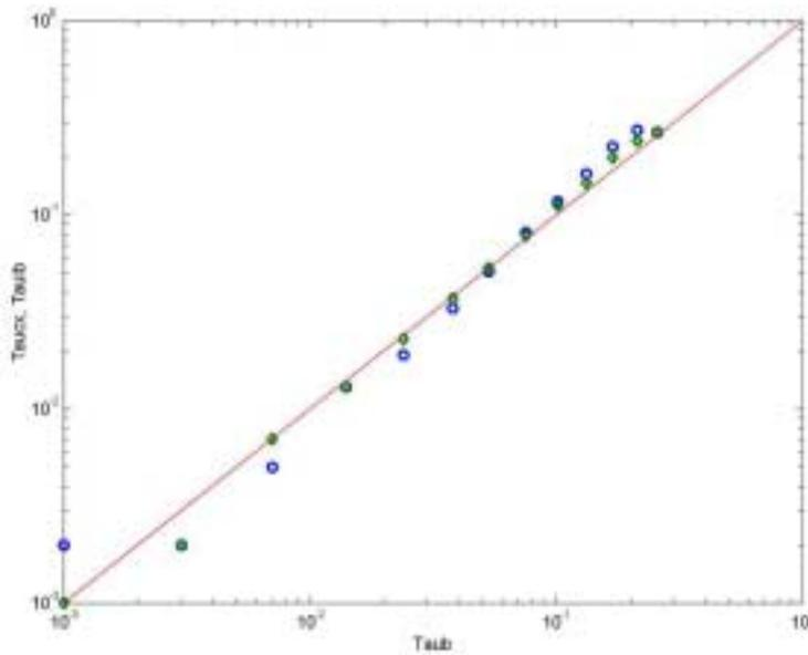
**Figure 3.** Comparisons of bulk and direct turbulence estimates of stress in 10-m neutral wind speed bins. The diamonds are inertial-dissipation estimates; the circles are covariance estimates.
