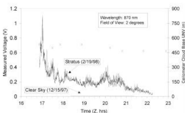
**Figure 4a.** Low stratus cloud NFOV measurements at 870 nm for a 5-hour period on February 19, 1998, at State College, Pennsylvania. Ceilometer cloud base heights at University Park airport (UNV) are also shown. The measured clear sky curve from Figure 3a is plotted for comparison.
