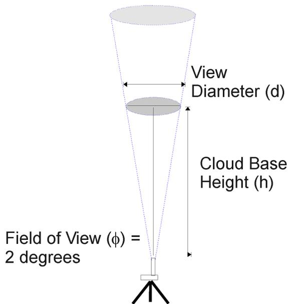
**Figure 2.** Instrument field of view geometry.
