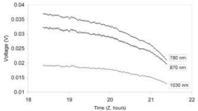
**Figure 3a.** Clear sky, zenith, NFOV measurements at 780 nm, 870 nm, and 1030 nm recorded at State College, Pennsylvania, on December 15, 1997.
