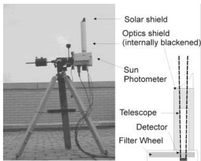
**Figure 1.** The modified setup of the PSU Sun Photometer to perform vertically pointing NFOV measurements.
