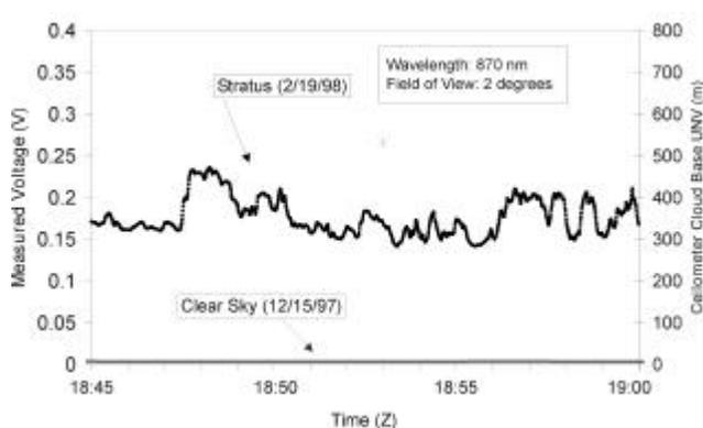
**Figure 4b.** A close up view of the February 19, 1998, NFOV measurements at 870 nm. The period shown here is from 18:45 Z to 19:00 Z.
