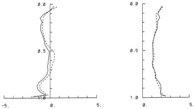
**Figure 5a** (left). Temperature, mean error through 10 days at Kingfisher, Kingman, and Pawhuska. Sigma level versus error (K). FDDA (solid), NOFDDA (dashed).
