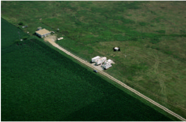
Figure 1. Aerial photograph of the LIFT site, near Urbana, IL. The lidars and wind profiler electronics are housed in the trailers. The wind profiler antenna surrounded by four Radio Acoustic Sounding System (RASS) speakers sits in the field. (For a color version of this figure, please see http://www.arm.gov/docs/documents/technical/conf_9803/cohn(2)-98.pdf .)
