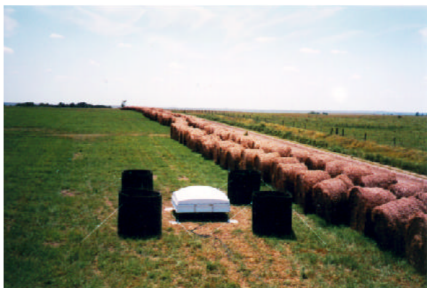
Figure 1. MAPR antenna and radioacoustic sounding system (RASS) deployed in the ARM Cloud and Radiation Testbed (CART) site, near Dexter, Kansas during BLX-96. (For a color version of this figure, please see http://www.arm.gov/docs/documents/technical/conf_9803/cohn(1)-98.pdf .)
