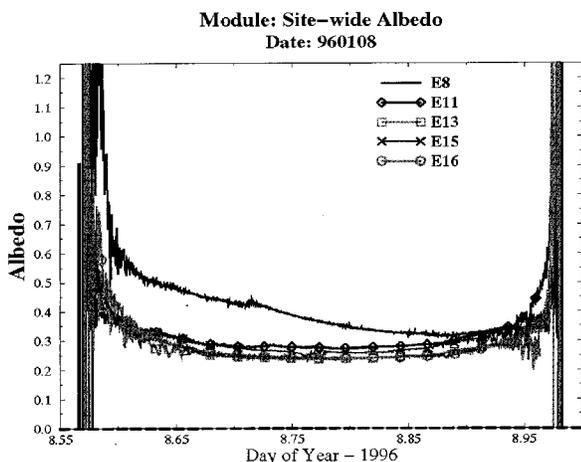
**Figure 2.** Albedo estimates displayed from across the Site reveal different behavior at one of the Extended Facilities, E8 (Ashton, KS). The data from E8 was found to be associated with melting snow-cover, while the other facilities had none.
