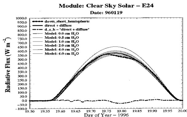
**Figure 1.** Display of SIROS derived estimates of the hemispheric broadband and modeled estimates for the Cyril, OK Extended Facility on January 19, 1996. 40  $W m^{-2}$  differences between the unshaded pyranometer (down\_short\_hemispheric) and that calculated from the direct and diffuse components are noted during mid-day.
