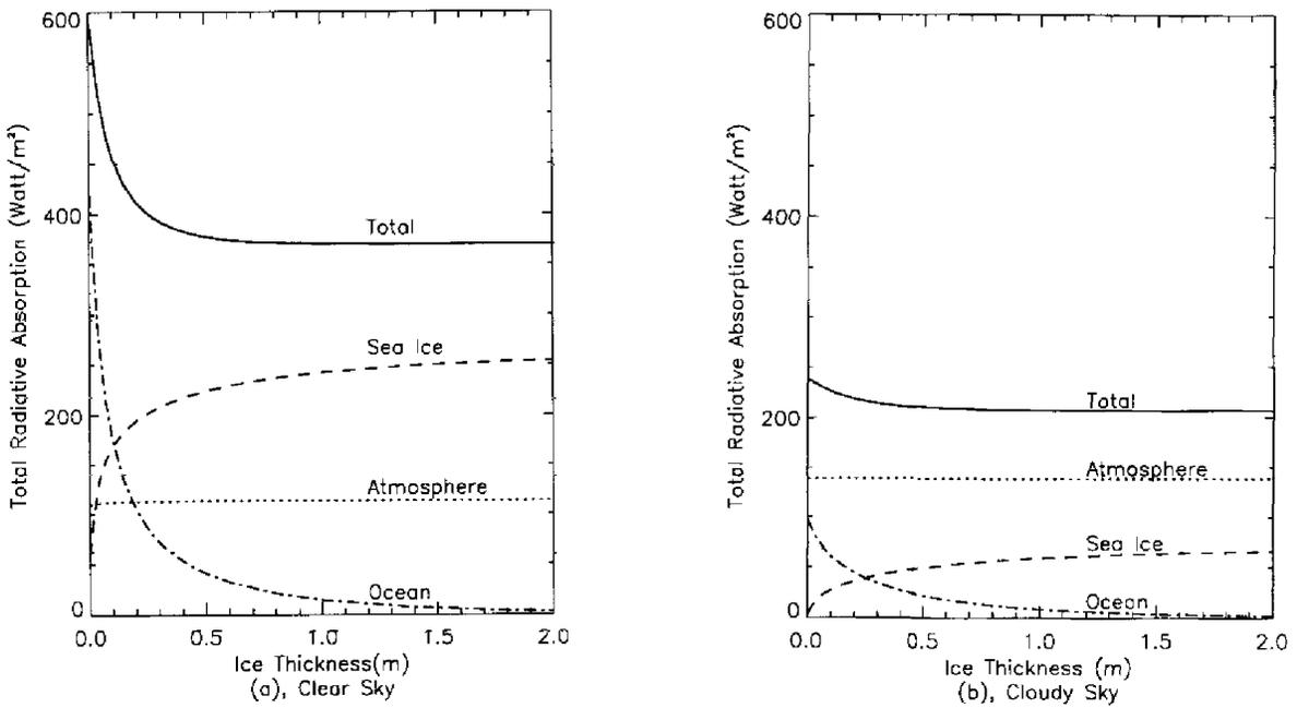
**Figure 5.** The distribution of total solar radiative absorption in the atmosphere, sea ice, and ocean system as a function of the ice thickness: a) under a clear sky; b) under a cloudy sky.
