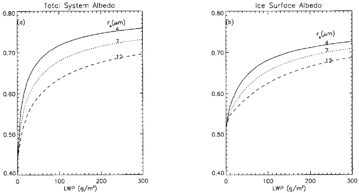
**Figure 4.** The total system albedo and the ice surface albedo as a function of cloud liquid water path (LWP). Labels represent the equivalent radii of clouds.
