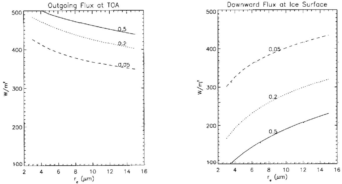
**Figure 1.** Shortwave flux as a function of the equivalent radius of cloud droplets: a) outgoing flux at the top of atmosphere; b) downward flux at the ice surface. Labels represent the liquid water content of the cloud.
