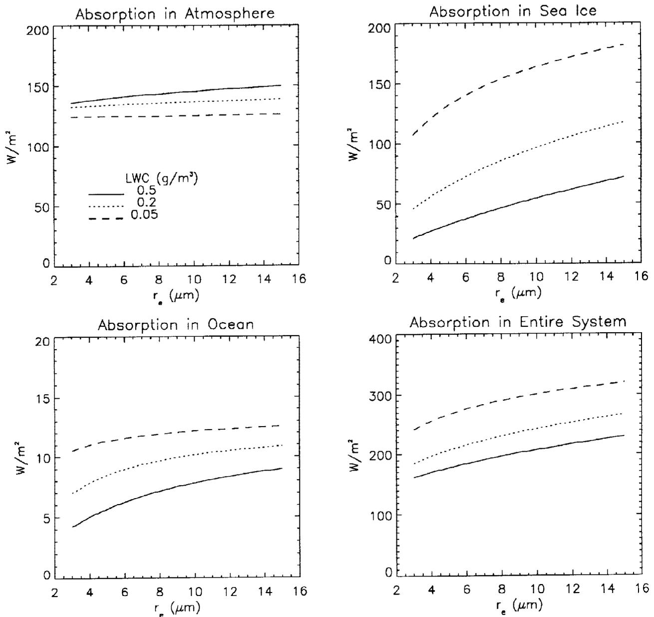
**Figure 3.** Absorption of solar radiation in various layers as a function of cloud equivalent radius.
