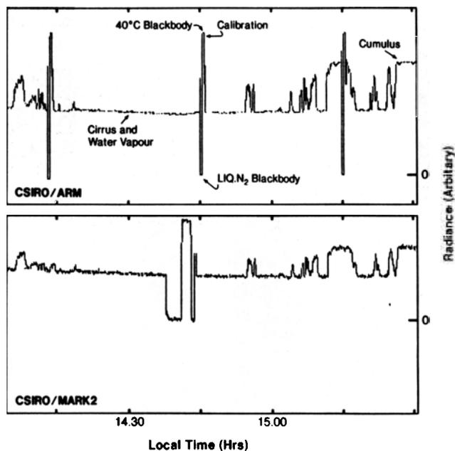
**Figure 5.** Comparison of the signal and noise output from the CSIRO Mark II and ARM radiometers for an observation period during PROBE. As the radiance is chopped against a 40°C blackbody, maximum negative signal is obtained when viewing a liquid nitrogen blackbody.
