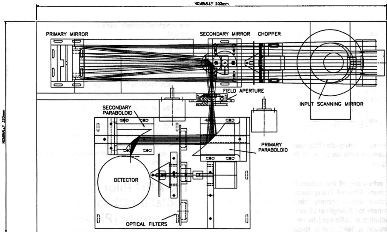
**Figure 4.** Schematic of the CSIRO/ARM filter radiometer optical system.
