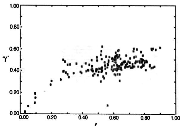
**Figure 3.** Integrated lidar backscatter ( $\gamma^1$ ) plotted against infrared emittance ( $\epsilon$ ) at  $10.84 \mu\text{m}$  for the same cloud as Figure 2.
