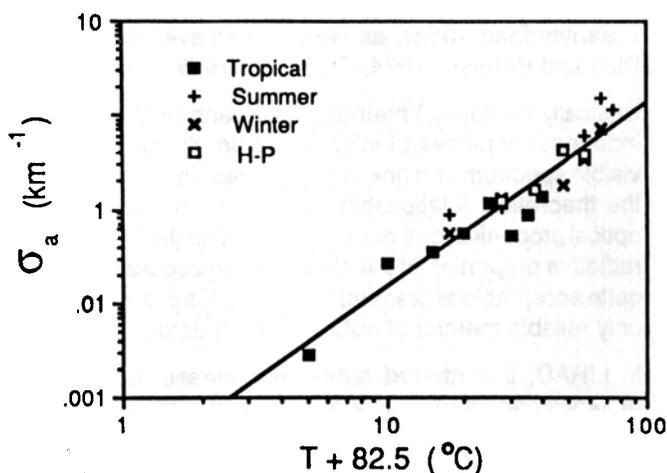
**Figure 1.** The variation in average infrared absorption coefficient ( $\sigma_a$ ) at  $10.84 \mu\text{m}$  wavelength with midcloud temperature ( $T$ ) for a year's data on mid-latitude cirrus (after Platt and Harshvardhan 1988).
