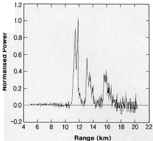
**Figure 6.** Lidar backscatter profile of tropical cirrus during PROBE.
