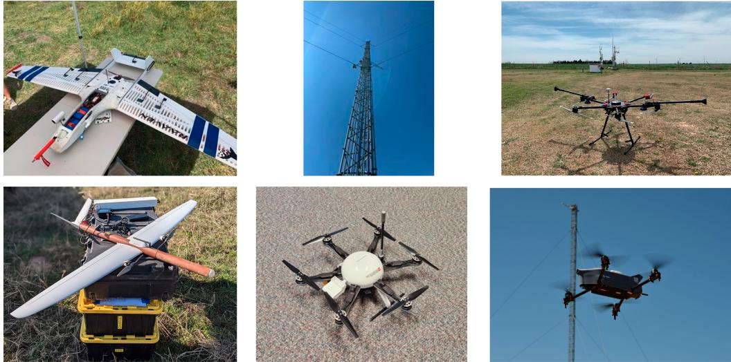
FIG. 1. Sensing systems used in this intercomparison, including (clockwise from top left) the University of Colorado RAAVEN, the ARM SGP 60-m tower, the University of Nebraska M-600, the University of Oklahoma CopterSonde 3D, the University of Nebraska Meteodrone, and the Black Swift Technologies S0.
