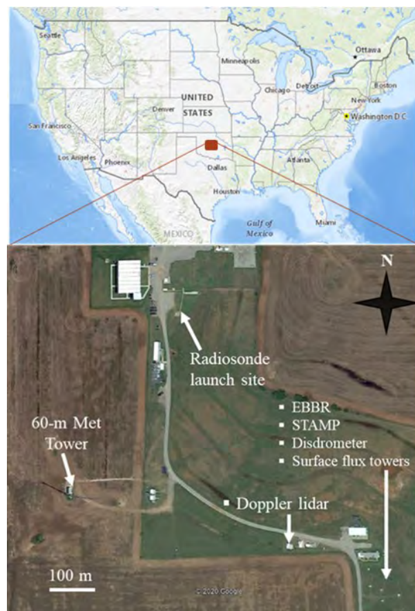
Figure 1. ARM SGP site C1 layout and instruments used in this study in Oklahoma, USA. Maps are extracted from © Google Earth and © Google Maps.
