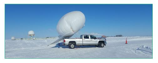
At the SGP, TBS are operated below clouds to perform vertical profiling—moving up and down within the boundary layer—and conduct sampling before and after convection. The maximum height allowed for TBS flights at the SGP is 1.5 kilometers (4,921 feet) above ground.
