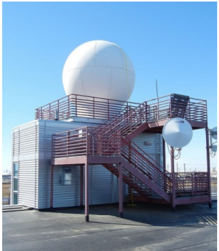
The ARM Climate Research Facility established climate research sites on the North Slope of Alaska to provide data about cloud and radiative processes in cold environments and high latitudes. Shown here is the X-band scanning ARM precipitation radar.
