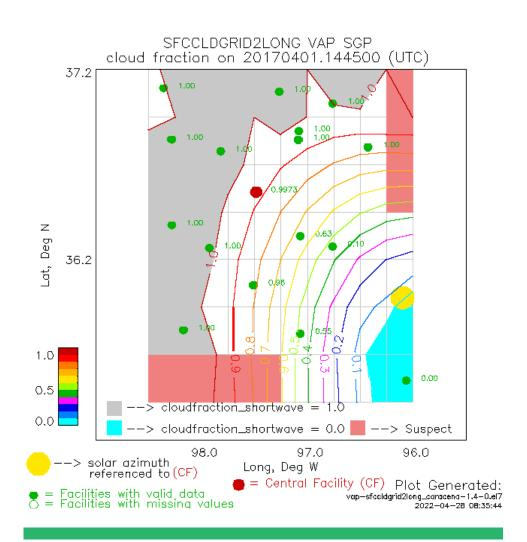
The figure illustrates SFCCLDGRID cloud fraction on the morning of April 1, 2017, when the Southern Great Plains (SGP) atmospheric observatory experienced partly cloudy conditions with clear skies to the east and overcast conditions to the west and north. The yellow ball represents the sun in the sky, the SGP Central Facility is noted in red, and other SGP facilities are noted in green.
