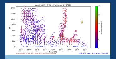
This figure from the EPCAPE campaign shows lowertroposphere 3D wind profiles retrieved by the Doppler lidar during Tropical Storm Hilary on August 20, 2023.
