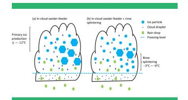
This schematic shows the proposed mechanisms of enhanced ice concentrations in the clouds observed over the Southern Ocean during ARM's MARCUS campaign. (a) Primary ice production occurs near the cloud top, which seeds the lower levels of the cloud, enhancing ice growth. (b) The process in (a) is modified by rime splintering, which leads to more but smaller ice crystals. (Copyrighted image from the journal.)
