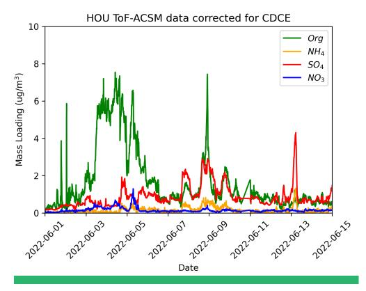
ARM also developed a VAP that corrects time-of-flight aerosol chemical speciation monitor data for compositiondependent collection efficiency, or the non-unity detection of particle mass by the instrument. This VAP brings the instrument data into better agreement with co-located aerosol measurements.
