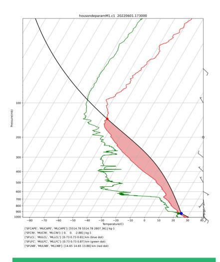
This skew-T plot shows the pressure and temperature recorded by a radiosonde launched June 1, 2022, at the ARM Mobile Facility site in La Porte, Texas, during the TRACER campaign. Red, blue, and green dots indicate different radiosonde parameters.
