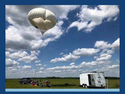
Researchers are using EMSL capabilities to study aerosol samples collected on tethered balloon system flights in Guy, Texas, during ARM's TRACER campaign.
