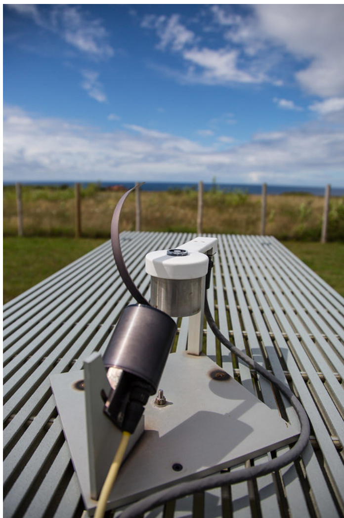
ARM updated multifilter rotating shadowband radiometers and other shortwave spectral instruments at its ground-based sites.
