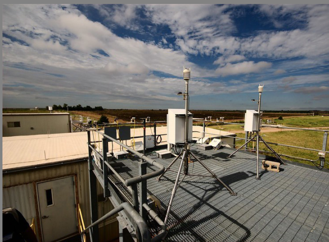
Radiometers and multiwavelength spectrometers at ARM's Southern Great Plains atmospheric observatory gather information about solar energy, a large variable in the earth system equation.
