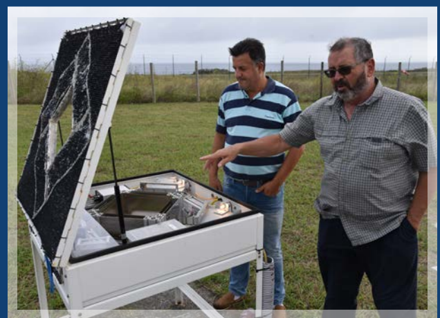
Paul Ortega, operations manager for ARM's Eastern North Atlantic atmospheric observatory, points to a two-dimensional video disdrometer as site technician Carlos Sousa observes.
