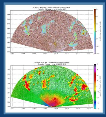
Plots of differential reflectivity (top) and reflectivity factor are shown from the X-band Scanning ARM Precipitation Radar on Graciosa Island in the Azores. Py-ART has a new experimental reader allowing the new format to be read.
