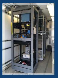
Ready for testing and calibration, instruments are racked inside the powered-up, air-conditioned ARM SeaTainer at Cape San Juan, Puerto Rico. The SeaTainer sits at the site of a long-term atmospheric observatory destroyed by Hurricane Maria. Photo is courtesy of John Ogren (retired from the National Oceanic and Atmospheric Administration).
