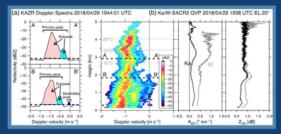
The data plots show that Doppler spectra are multimodal, making it possible to identify different particle populations that coexist in one radar sampling volume. The tall (primary) peak at the top left, for example, shows how cloud reflectivity is dominated by ice particles and not cloud droplets. The color-shaded profile plot in the center offers another view of variances in reflectivity from different populations in the column above the radar. (Copyrighted image from the journal.)
