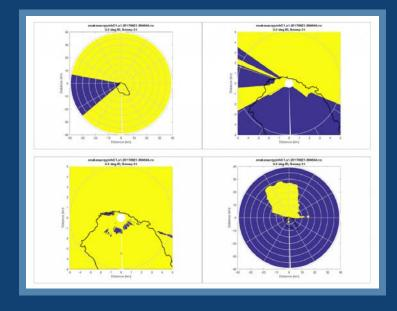
The example masks shown here are associated with the ENA scanning radars and are for plan position indicator (PPI)-type scans. The masks are also applied to range height indicator (RHI)- and vertically pointing (VPT)-type scans. The scan types are denoted by the datastream name, which is part of the file name identified above the plot.
