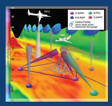
In this representation of MC3E, research aircraft fly above and within the clouds, radar systems scan through the storm from multiple locations, and additional ground-based instruments measure surface precipitation and wind speed. Image courtesy of Brookhaven National Laboratory.
