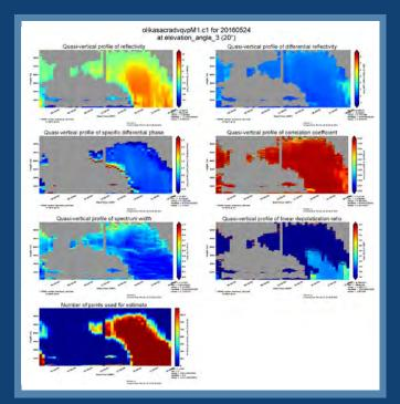
The Scanning ARM Cloud Radar ADVance Quasi-Vertical Profile (SACR-ADV-QVP) provides a quasi-vertical representation of azimuthal averaged polarimetric variables.
