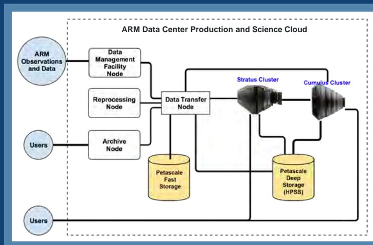
ARM’s new high-performance computing facility integrates multiple levels of computing resources and storage systems.
