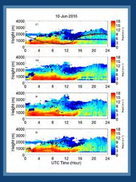
Time-height images are shown here of the wind speed at a uniform 10-minute and 50-meter resolution from the radar wind profilers at the SGP atmospheric observatory.
