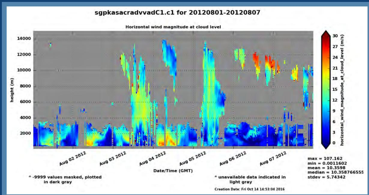
In 2017, evaluation data using the SACR-ADV-VAD VAP were produced for August 2012 at the SGP observatory. The first seven days of horizontal wind speed and direction at cloud level are shown here.
