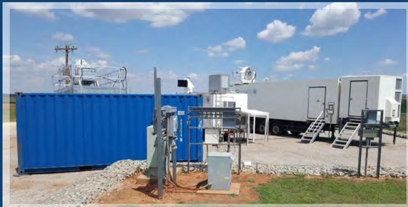
LAFE benefited from a variety of specialized scanning equipment, including the NOAA Doppler lidar DALEK (on the blue container), University of Hohenheim scanning temperature lidar (central white trailer), and University of Hohenheim scanning water vapor differential absorption lidar (trailer on the right).
