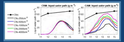
No matter the aerosol number concentration (CN in the legend), results from the cloud-resolving model (CRM) and earth system model (CAM) could not match real-world observations for how clouds and aerosols react to influence cloud lifetimes.
