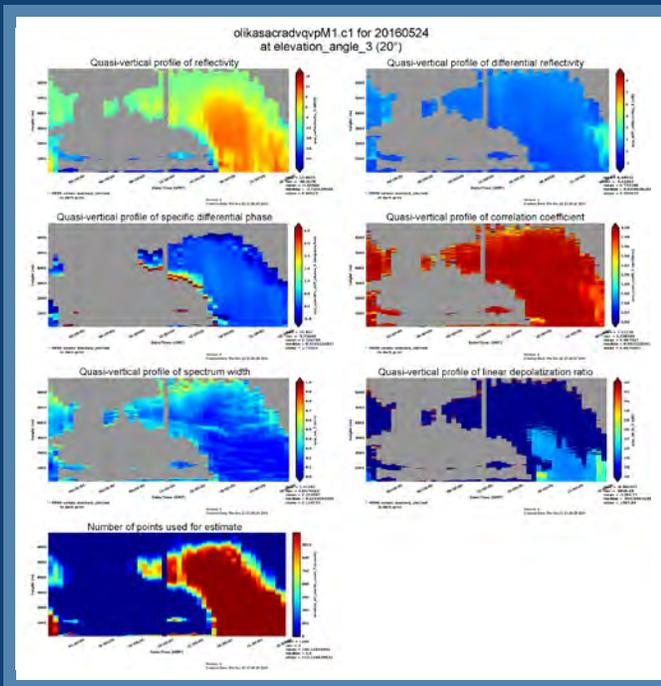
The Scanning ARM Cloud Radar ADVance Quasi-Vertical Profile (SACR-ADV-QVP) provides a quasi-vertical representation of azimuthal averaged polarimetric variables.
