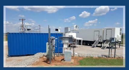
LAFE benefited from a variety of specialized scanning equipment, including the NOAA Doppler lidar DALEK (on the blue container), University of Hohenheim scanning temperature lidar (central white trailer), and University of Hohenheim scanning water vapor differential absorption lidar (trailer on the right). Image courtesy of Volker Wulfmeyer, University of Hohenheim.
