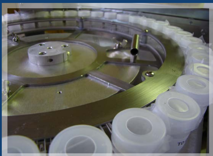
Data gathered during the CARES campaign, from state-of-the-art instruments on the ground and in the air, such as this particle in liquid auto sampler, or PILS, are still being used by researchers to learn more about aerosols.
