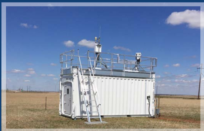
Situated on top of a shipping container, this three-channel microwave radiometer (left) is one of the new profiling instruments added to the Southern Great Plains atmospheric observatory.
