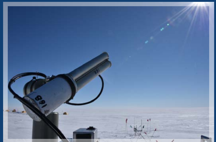
A sun photometer measures direct solar irradiance and sky radiance at the Earth's surface from West Antarctica.
