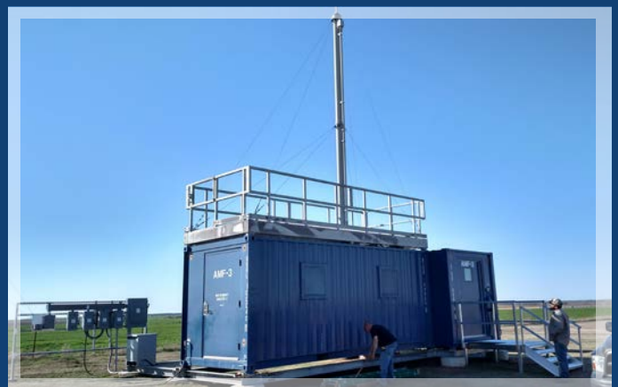
Before deploying to the Alaskan North Slope, this Aerosol Observing System for the third ARM Mobile Facility made a stop at the Southern Great Plains atmospheric observatory for testing.
