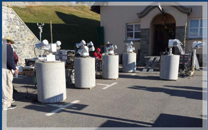
Maintaining data quality for the measurements from radiometers requires accurate and regular recalibration traceable to the World Radiometric Reference, the international standard of solar radiation measurement.
