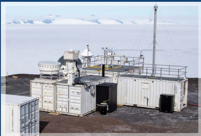
From McMurdo Station, the second ARM Mobile Facility gathers sophisticated data with cloud radars and high spectral resolution lidar and a complete aerosol suite.
