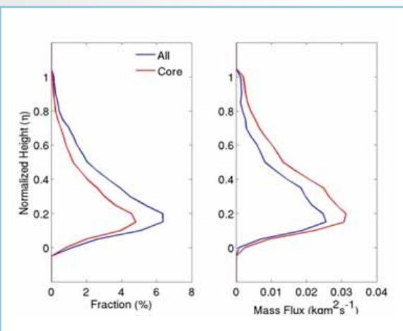
Profiles of cloud fraction (left) and vertical mass-flux (right) for 557 individual trade cumulus clouds (114 hours), derived from the 94-GHz vertically pointing radar during the CAP-MBL campaign. Profiles from vertically moving core regions (red) and for the entire cloud (blue) are shown.
