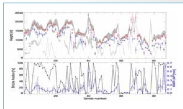
The upper panel shows cloud boundaries (base from the ceilometer [blue] and top from the WACR [red]) averaged over 2 hours surrounding sounding times, superimposed on the soundings inversion and transition layers (dark and light shadings, respectively). The lower panel shows the fraction of the 2 hours that experienced drizzle (black) and the 2-hourly averaged LWP from the MWR (blue). In both panels, vertical lines represent the 2-hourly standard deviations of the measurements.
