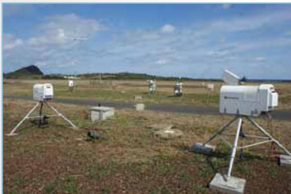
Microwave radiometers deployed in the Azores gathered measurements of marine boundary-layer cloud properties, such as water vapor and liquid water content.
