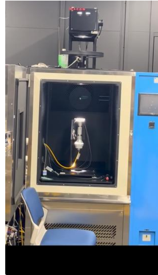
Example image on how the temperature chamber will be used to characterize radiometers
