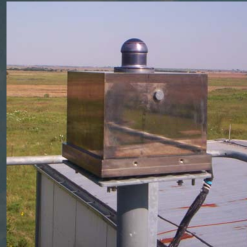
Blue Sky Imaging All Sky Thermal Infrared Camera (ASTIC)
