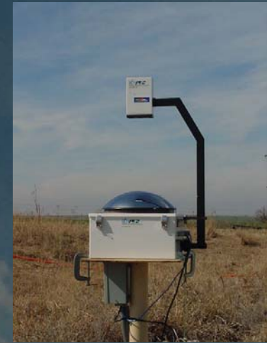
Blue Sky Imaging All Sky Thermal Infrared Camera (ASTIC)
