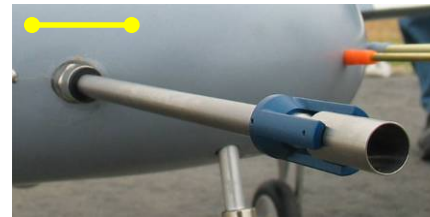
Aerosol inlet & splitter (150 g) → unbiased aerosol sampling
