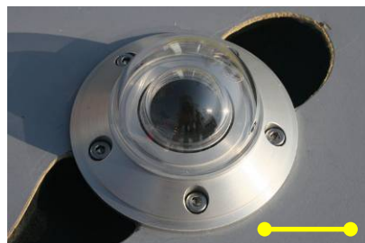
Pyranometer (190 g) → irradiance 0.3 - 2.8 \mu\text{m}
