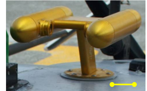
Cloud Droplet Spectrometer (1.4 kg) → distr. 1 < D < 50 \mu\text{m}
