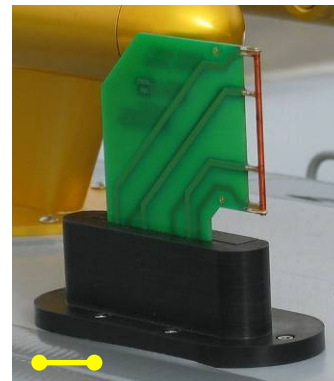
LWC probe (450 g) → Cloud water ( \text{g m}^{-3} )
